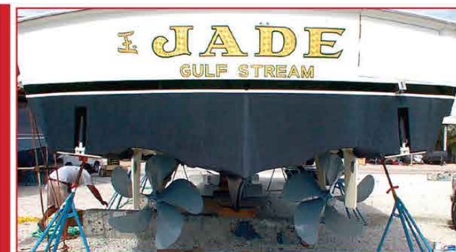
JADE WITH FRESHLY COATED PROPS, SHAFTS AND SCREWS
