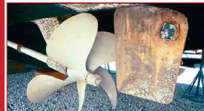
COATED PROP, SHAFT AND NUTS AFTER 12 MOS. OF USE
