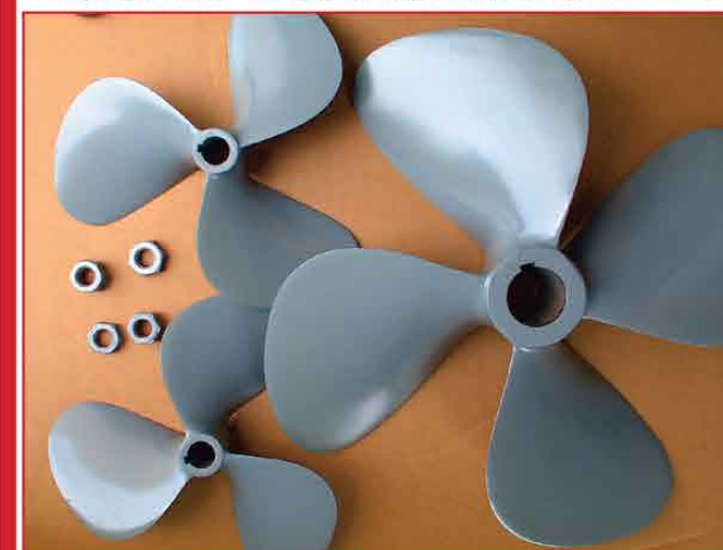
COATED PROPS READY FOR RE-INSTALL
