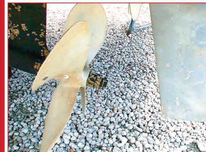
COATED PROP & RUDDER AFTER 20 MOS. OF USE
